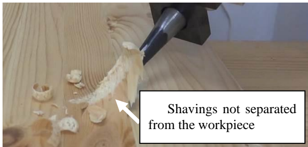
Figure 2. Excessive workpiece carving with improper machining path
